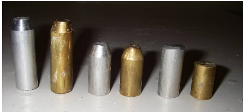
Figure 10: Cargo rounds types from left to right; Long Al, Long Br, Short Al, Short Br, Al b2, and Br b2
