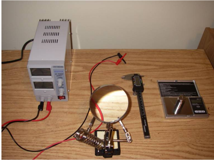
Figure 19: Power supply, calipers, magnifying glass, and scale used for characterizing motors pre and post shock
