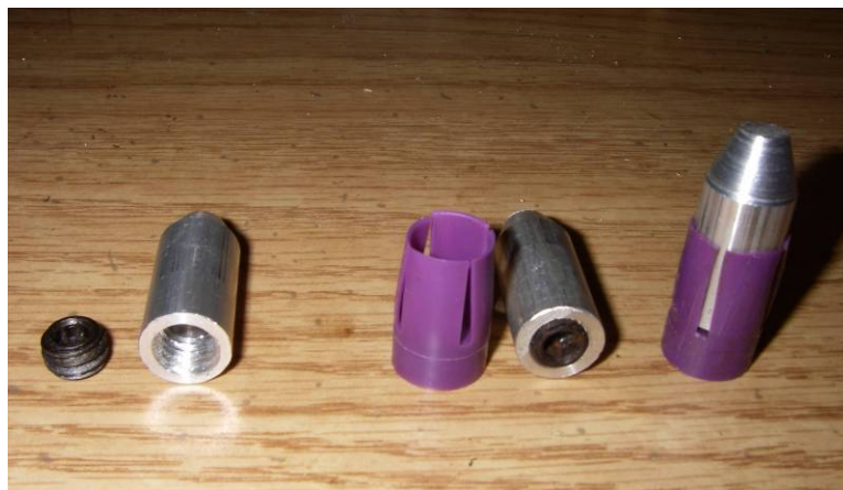
Figure 11: Assembly procedure for sabot launched cargo rounds
