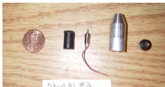
Figure 16: RC helicopter tail motor shown next to short aluminum cargo round
