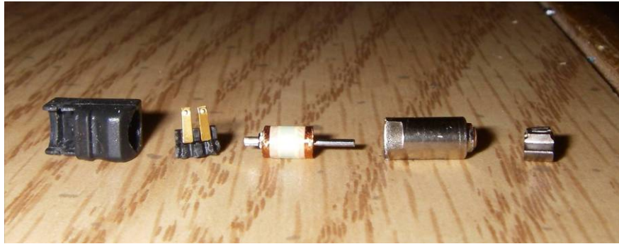
Figure 37: Components of Small Black Pager motor type from left to right; rubber casing, rear contact assembly, axle/winding assembly, case, and vibration weight
