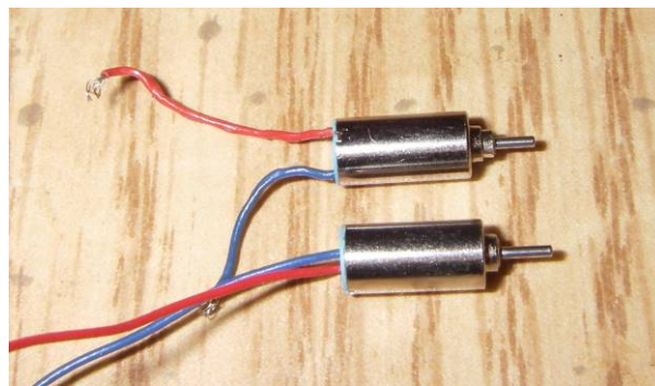
Figure 32: Comparison of unfired (bottom) and fired (top) Short IR type motors indicating compression of shaft into casing by launch loads.
