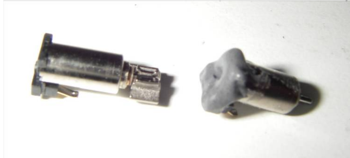
Figure 39: Short Silver type motor, launch 29, with JB weld sealed rear portion (right) versus original condition (left)
