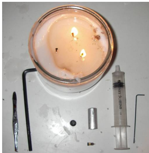
Figure 23: Setup for wax encapsulant mounting of motors in cargo rounds
