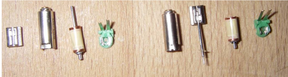
Figure 33: Disassembly of Long Silver motors with axle intact (left) and fore/aft section separated (right)
