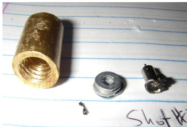
Figure 41: Short Silver type motor showing damaged rear portion and broken off plastic piece in foreground, launch 35
