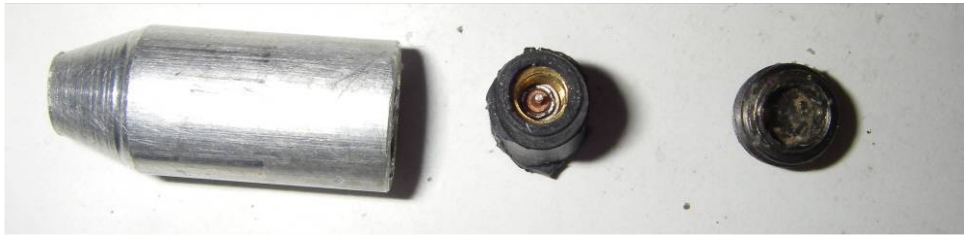
Figure 22: Motor mounted in rubber well nut showing motor housing resting on well nut metal end with axle pointing outwards
