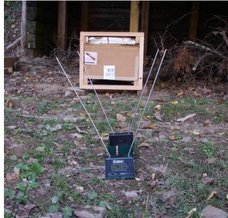
Figure 18: Ballistics chronograph for measuring muzzle velocity setup in front of soft capture device
