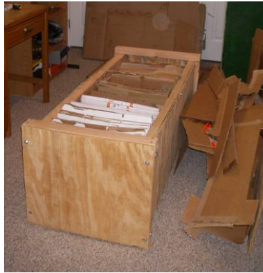
Figure 7: Soft capture device with top removed showing cardboard panels
