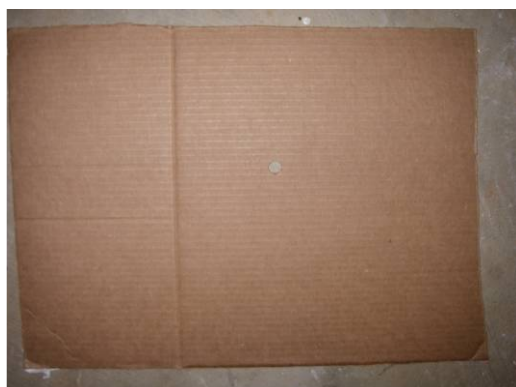
Figure 57: Yaw card for launch 36 with Short Br b2 #2 cargo round
