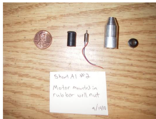
Figure 31: Short IR type motor prior to insertion in rubber well nut for launch number 5
