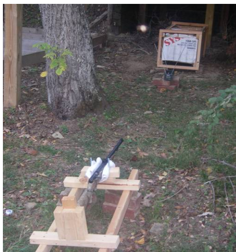
Figure 17: .54 muzzleloader and rifle stand used for launching cargo rounds, soft capture device and chronograph in background
