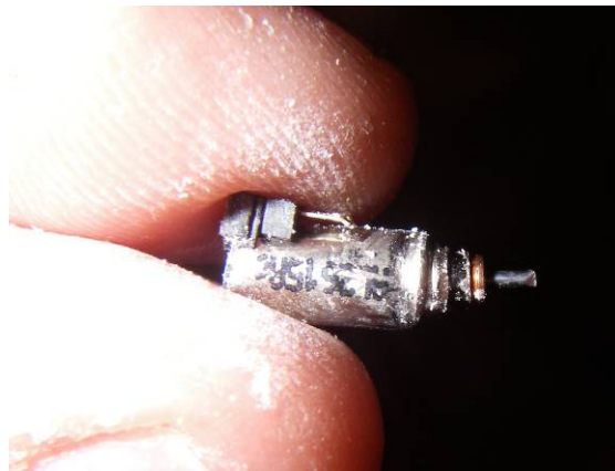
Figure 43: Launch 39 result showing ejection of axle and windings due to violent deceleration
