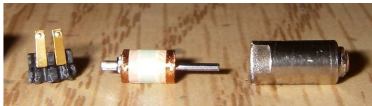
Figure 46: Components of Short Silver type motor from left to right; rear contact assembly, axle/winding assembly, and case
