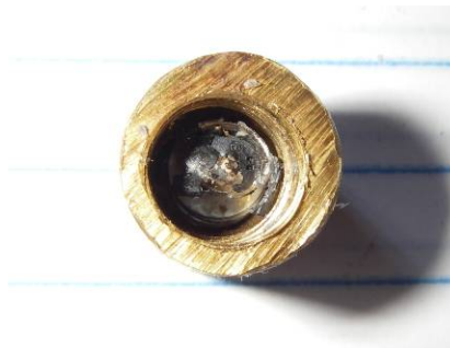
Figure 40: Short Silver type motor after launch before being extracted from cargo round, launch 35
