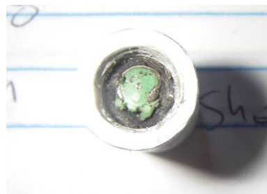
Figure 35: Long Silver type motor with rear end deformed due to setback loads in launch 40
